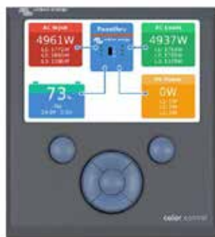
Color Control GX, showing a PV application
